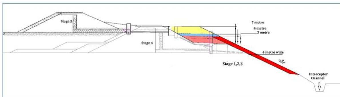
**Figure 1-1: Cross section of existing embankment walls and proposed buttress.**
